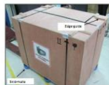
Erected pack with skid-mate and edge guide to improve protection and shock absorption.
